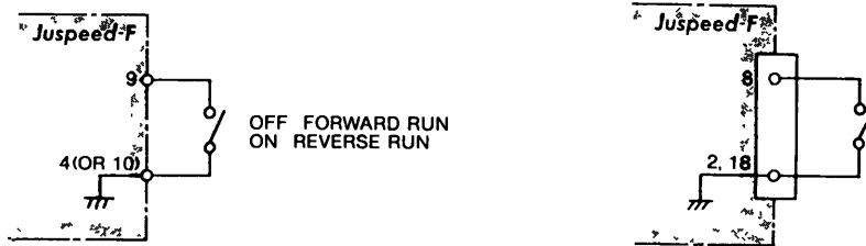
(a) Terminal Block TM2 Used
